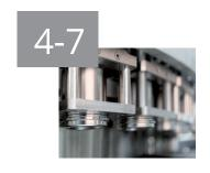
DESCRIPTION OF THE CAN FILLER WITH A PERFORMANCE LEVEL OF UP TO 3,500 CANS PER HOUR
