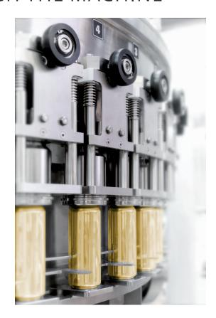
The entire drive system of the machine is based on decentralised SEW Moviaxis servo drives with electronic synchronisation. This enables the deployment of the non-table-design of the machine frame and thereby achieving an excellent cleanability of the external surfaces that are minimised and sloped and offer easy access to individual parts of the machine during its maintenance.
