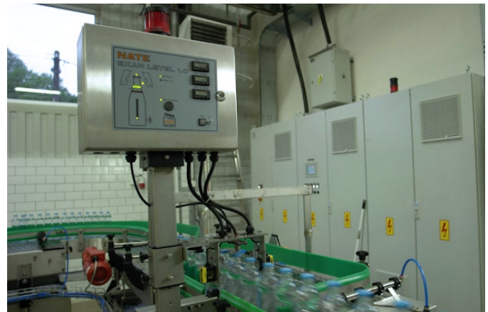
Exan Level (inspection of the drink level and presence of caps behind the filling machine)
