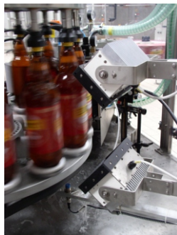
Exan Label CCD (inspection of the presence of labels - built into the labelling equipment)
