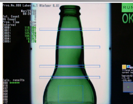
Exan Sort CCD equipment monitor (inspection of shape and colour of bottles)
