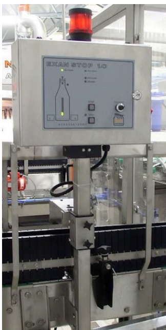
Exan Stop (inspection of residual liquid before filling)
