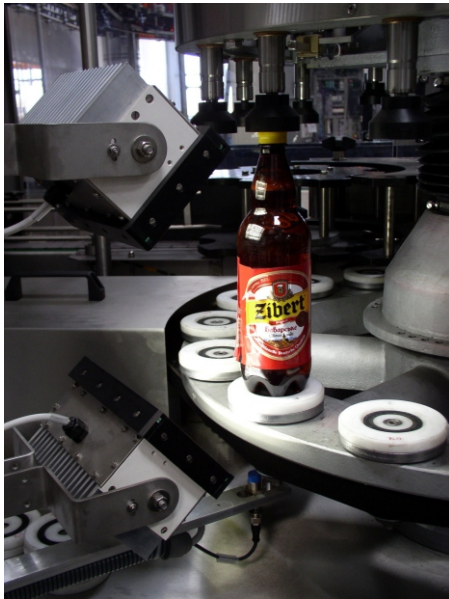
Exan Label CCD (inspection of the presence of labels - built into the labelling equipment)
