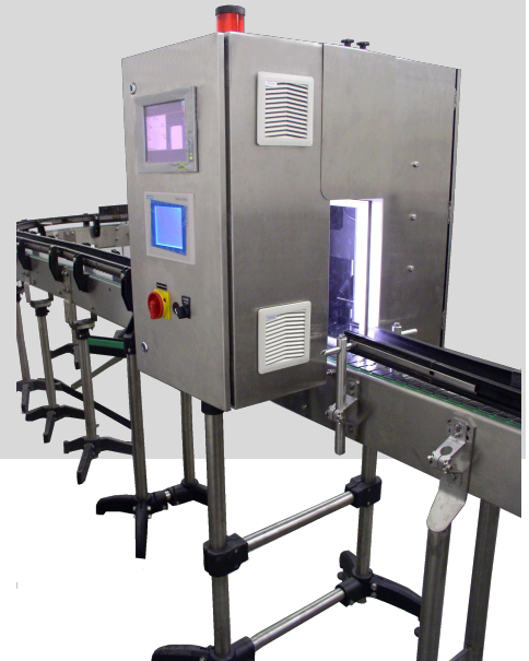
Exan View (inspection of the level, caps and labels of PET bottles)
