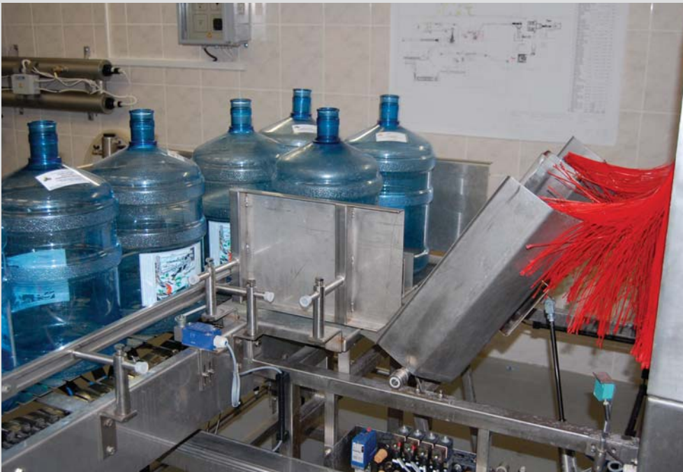
Line No. 5 – Entry of 18.9 l (5 gallons) containers in the washer
