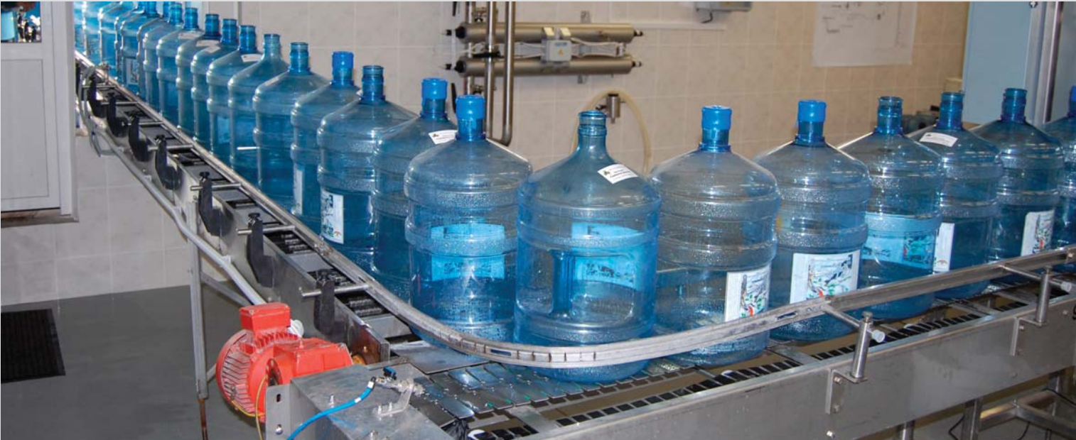
Line No. 5 – Conveying 18.9 l (5 gallons) containers to the washer
