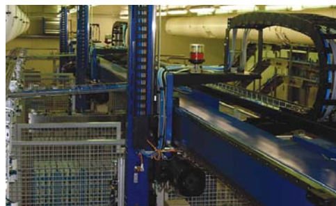
Palletisation cartons: performance of 1500 cartons per hour.
