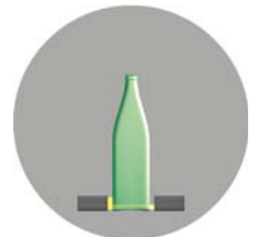
Checking for residual liquid by the high-frequency method
