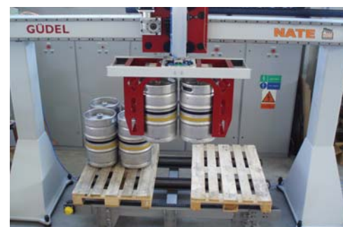
Palletisation / depalletisation of KEG barrels, with performance of 120 KEGs / hr.
