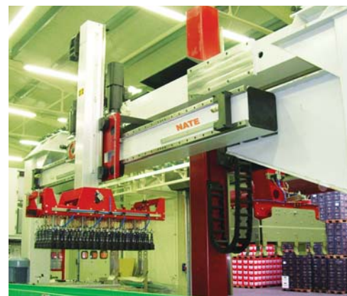
Inserter of bottles - GÜDEL manipulator with double-axis linear guidance.
